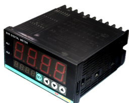
Temperature Indicator (Reference no: 9000-01)
